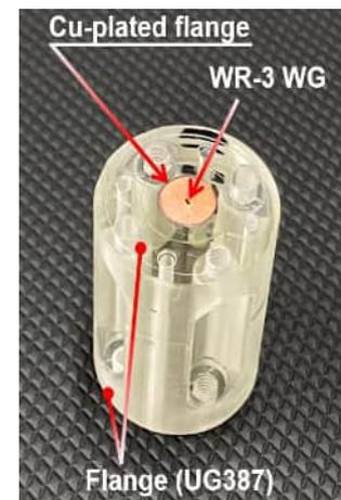
Fig. 1 RECILS-printed straight waveguide for 200–400 GHz
