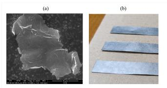
Figure 1. The material under investigation: (a) a single GNP flake (the scale is  $10 \ \mu m$ ).; (b) macroscopic GNP thin films.
