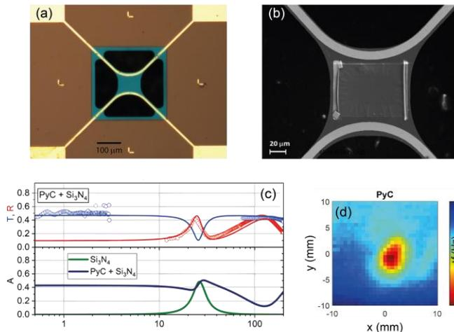
Fig. 1. (a): Microscope image of a typical TMB. (b): SEM of the PyC absorber integrated in the TMB. (c): Transmission and reflection spectra of a PyC film on Si<sub>3</sub>N<sub>4</sub>. Bottom panel shows estimated absorption obtained adding a 18 nm PyC film on the bare silicon nitride. (d): Beam profiling of the 140 GHz source using a PyC-TMB.
