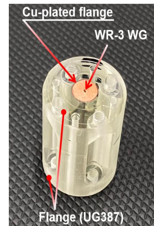
Fig. 1 RECILS-printed straight waveguide for 200–400 GHz
