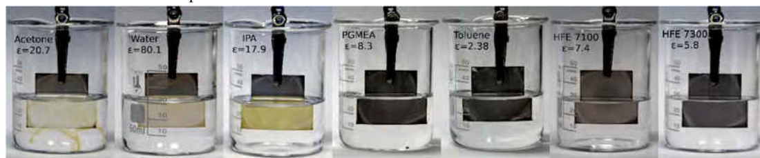
Fig. 1. Solvency tests of \text{CH}_3\text{NH}_3\text{PbI}_3 in various solvents with different polarity. Photographs of the samples were taken after 10 min immersion (10 seconds in case of acetone).
