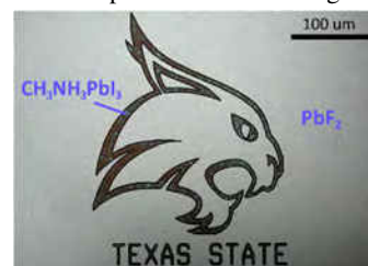
Fig. 2. High-Resolution Patterning of Organohalide Lead Perovskite Pixels for photodetectors using Orthogonal Photolithography
