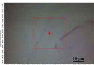
Fig. 1. Optical image of drop-casted graphene flakes.
