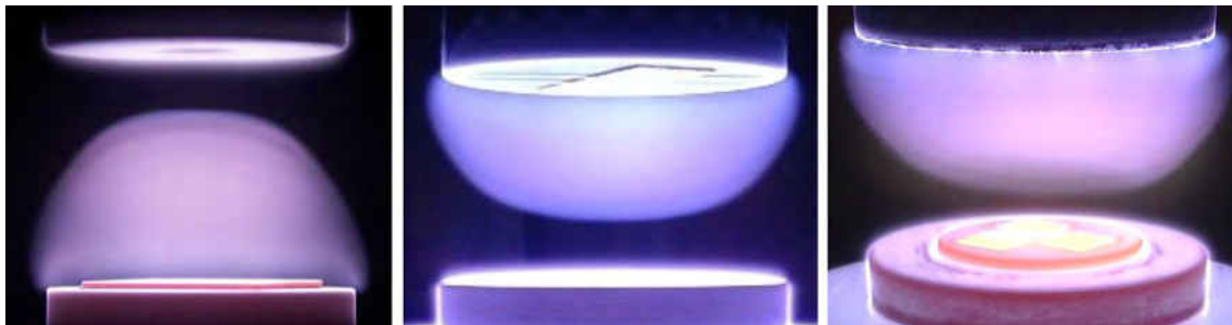
Fig. 1. Photo images of the DC CVD activation region in case of: standard (left), inverted gravity (middle) and inverted electric field (right) configurations.
