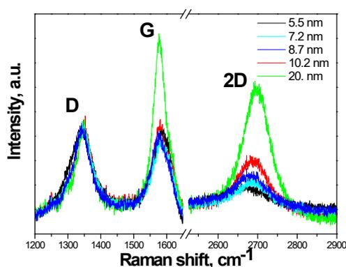
**Figure 1** Raman spectra of MWNT with diameters fixed by HRTEM images (series 1).
