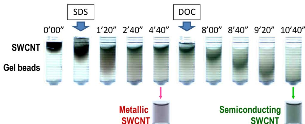
Figure 1. Pictures of continuous agarose gel beads separation of SWCNTs.
