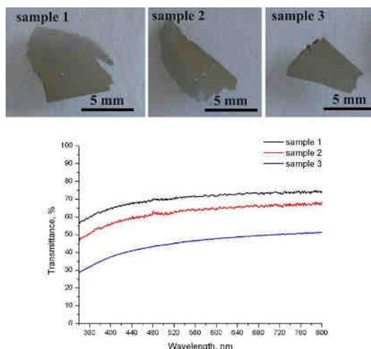
Fig.1. The optical absorption spectra of the different samples. The samples with numbers 1, 2, 3 contain 13, 17 and 26 graphene layers, correspondingly.
