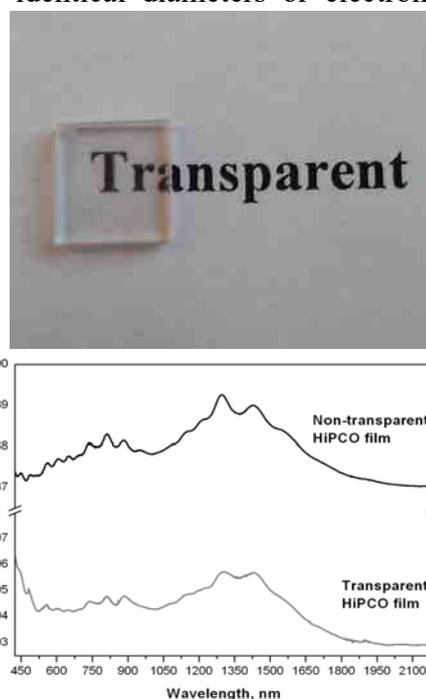
**Fig.1.** A photo of the transparent metallic SWNT film deposited on quartz substrate and UV-VIS-NIR optical absorption spectra of transparent and non-transparent films.
