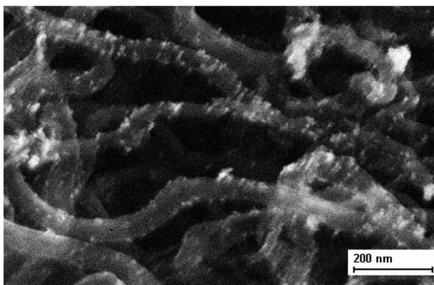
used for Raman measurements. Also sample functionalized by Pt-catalyst nanoparticles with the size distribution 3 - 6 nm was studied.
