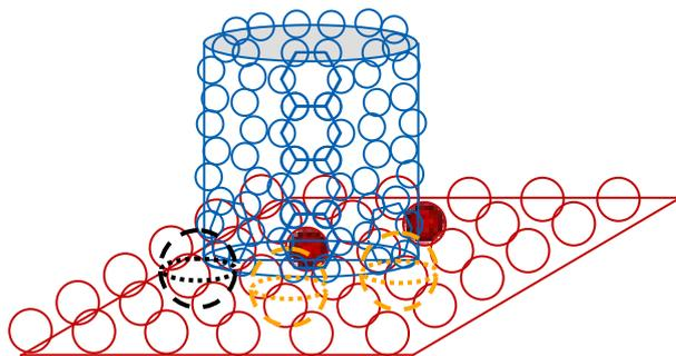
Figure 1. Model of ‘active bonds’ for CNT-Metal Interconnect
