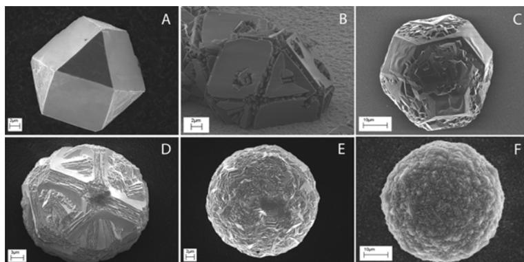
SEM images of CVD diamond crystallites grown at different methane concentrations
