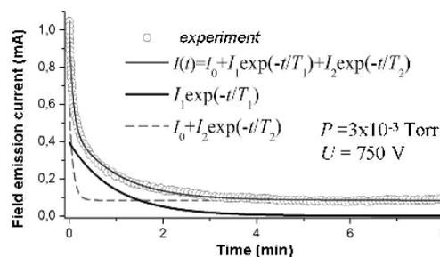
**Fig. 2.** Experimental FE current dependence on time at  $3 \times 10^{-3}$  Torr and the approximation curves.
