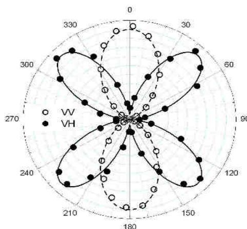
Fig.1. Intensity of Raman line  $1592\text{ cm}^{-1}$  depending on the angle between the incident light polarization and the nanotube axis.
