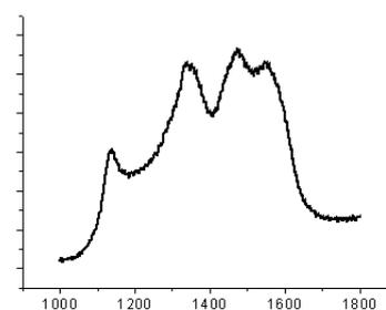
Fig 2. Raman spectrum of UNCD film
