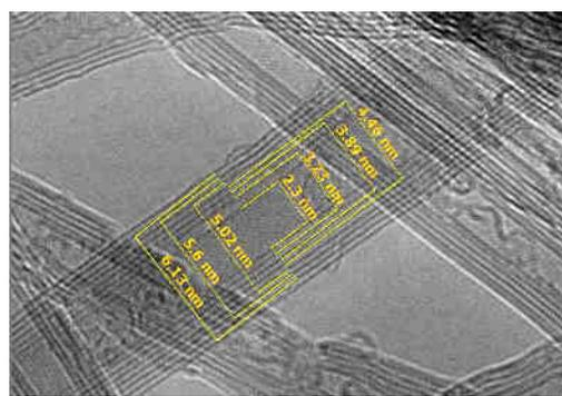
Fig. 2. HRTEM image of the CNT grown by the catalyst free CVD.
