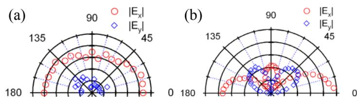
Fig. 2: Results of pump polarization dependence of THz radiation from (a) Sample A, and (b) Sample B.
