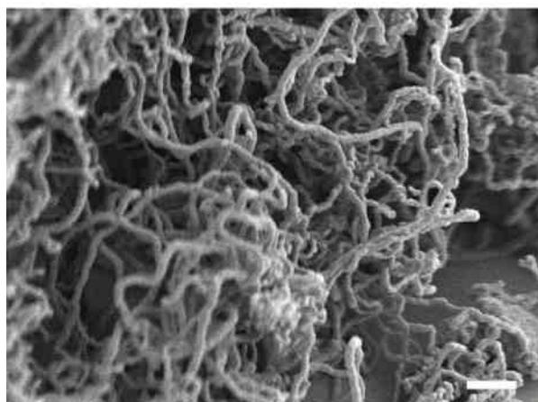
Figure. SEM image of cement particles covered by CNFs synthesised in a fluidized bed reactor at 550 °C in CO and C<sub>2</sub>H<sub>2</sub> atmosphere (bar scale is 200 nm).
