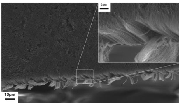
Fig. 1. SEM images of the CNT forest, obtained by the catalyst free CVD.
