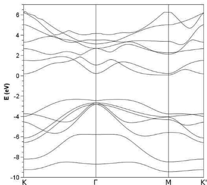
*Fig.1. - Calculated energy bands for the single GaSe tetralayer.*
