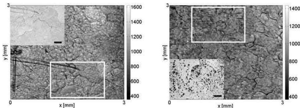
Figure 1. Glossmaps of two nanographite films on Ni substrates. One can observe that average gloss of the sample (a) is about 200 Gloss Units (GU) higher than that of the sample (b) indicating the difference in the nanographite film quality. Insets show images of the selected areas obtained with optical microscope (inset scale bar is  $200 \mu\text{m}$ ).
