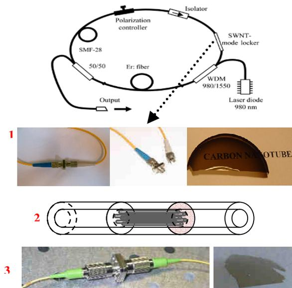
**Figure 1.** The nanocarbon-based saturable absorbers for Er fiber lasers in form of: **1** – a polymer film with embedded SWNTs, **2**- a piece of a holey fiber with a thin film of SWNTs on the hole walls(after drying) , **3**- a film containing a few layers of graphene.
