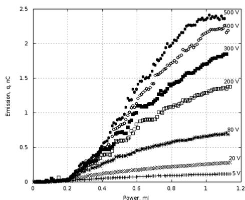
Fig. 1: Emitted electric charge as function of the laser pulse energy for different applied voltage
