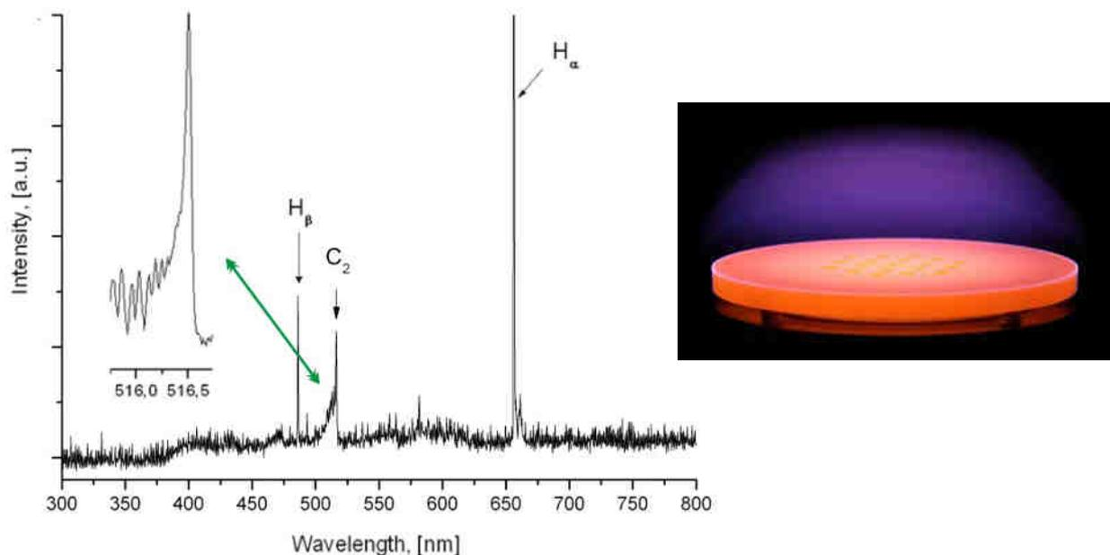
Figure 1. Typical emission spectra for hydrogen-methane gas mixture and photograph of the plasma above Nb anode plate
