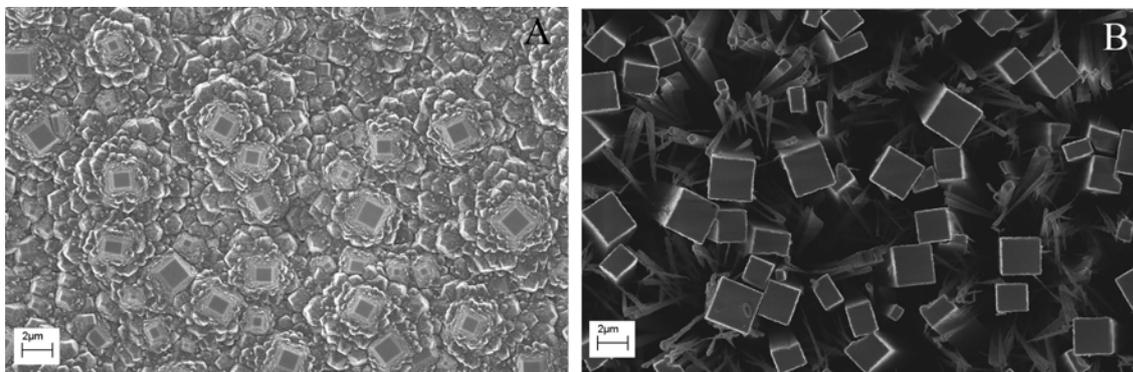
SEM images of CVD diamond film: (A) before and (B) after thermal oxidation
