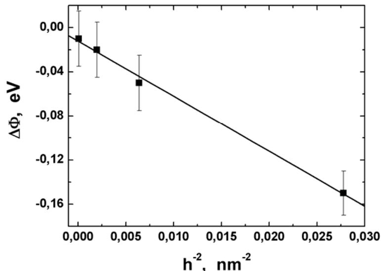
Fig. 1. The work function of electron variation  $\Delta\Phi$  vs. the film thickness  $h$  plot.
