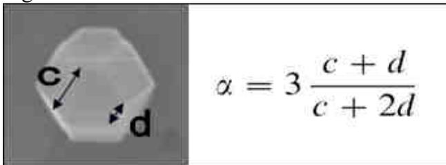
Figure 1. SEM image of a diamond crystallite on the silicon substrate and formula for calculation of parameter  $\alpha$ .
