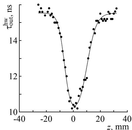
Experimental results presented in Figure show that the scanning a cuvette with aqueous suspension of multiwalled carbon nanotubes along the optical axis is accompanied by smooth change of nanosecond laser pulses duration transmitted through suspension. At  $z = 0$  the duration of transmitted laser pulse is  $\tau_{\text{out}}^{\text{hw}} \approx 10$  ns. Thus incident YAG: Nd<sup>3+</sup>- laser pulses of 16 ns duration have been smoothly adjusted in the range of 10 - 16 ns.
