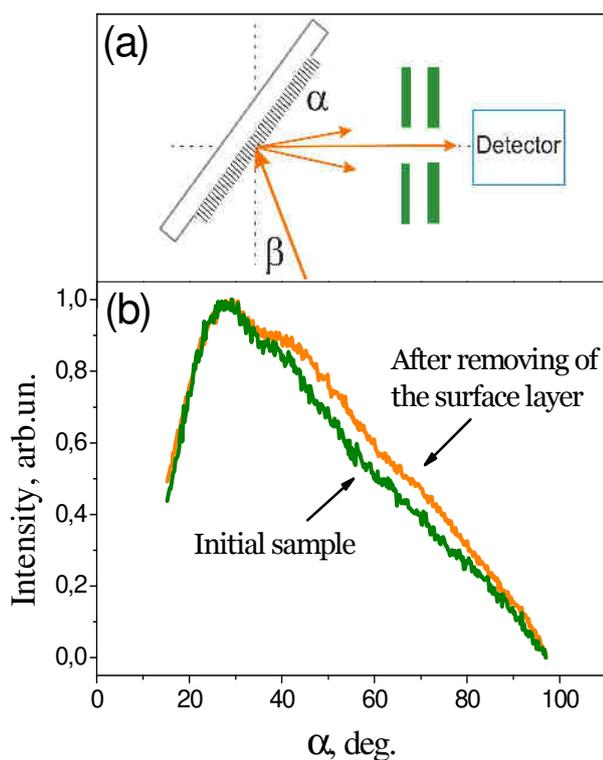
Fig.1. (a) Optical scheme of experiment; (b) X-ray scattering curves of initial sample and after removing of the surface contamination.
