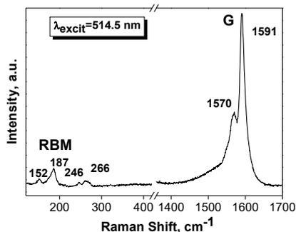
**Fig.1.** Raman spectra of SWCNTs on quartz surface registered with a laser excitation 514.5 nm.
