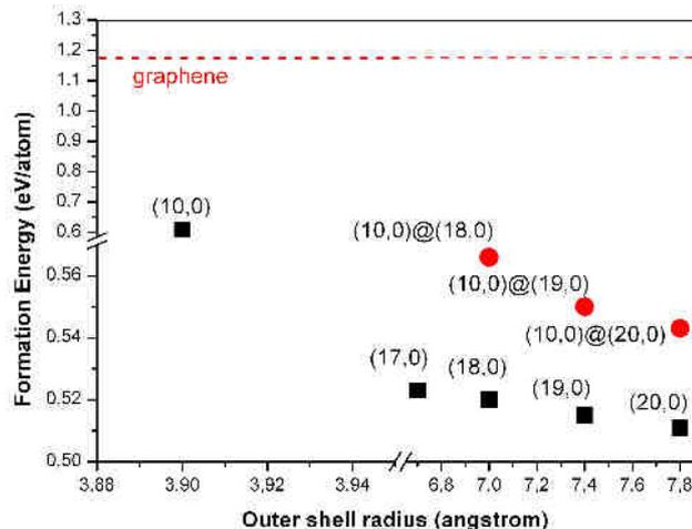
Fig. 1. Formation energy per atom as a function of nanotube radius.
