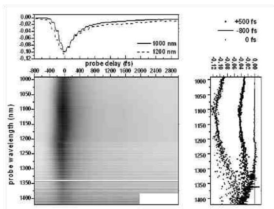
pump-probe measurements of light-induced absorbance change in thin films were carried out with 150 fs laser in near-IR spectral range (probe range: 900-1600 nm, pump range: 1100-1650 nm). Dependences of saturable absorption signal level and relaxation dynamics on pump wavelength, energy and number of graphene layers are obtained.
