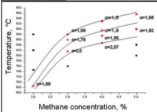
Figure 2. Diagram of dependence of  $\alpha$  on the substrate temperature and the methane concentration in the gas mixture.
