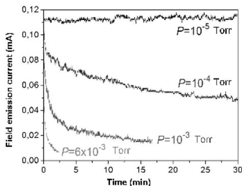
**Fig. 1.** FE current dependence on time at different pressure values (at dc voltage of 1200 V).
