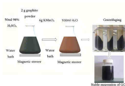
Fig. 1. Illustration of the preparation of GO
