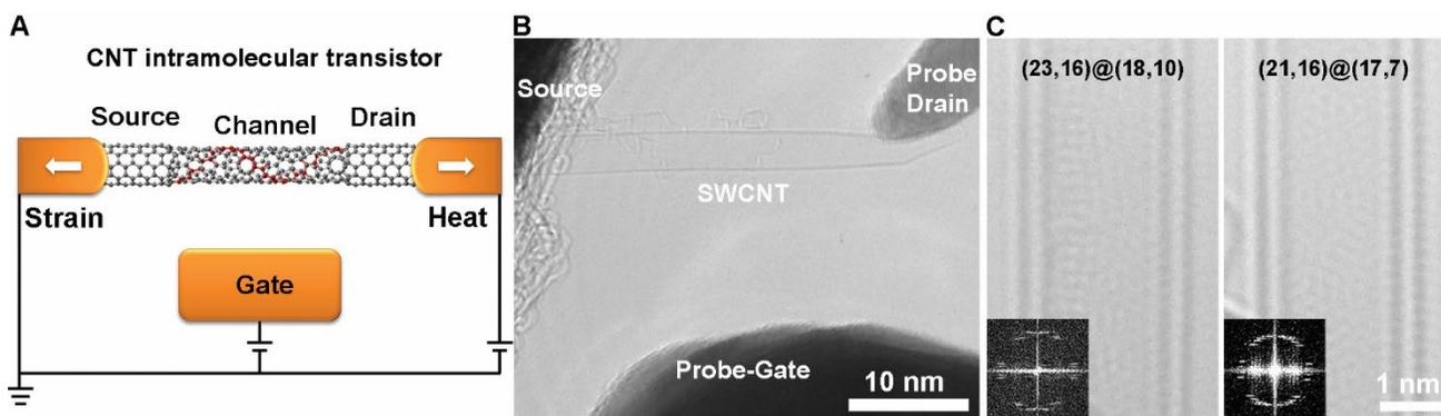
**Fig. 1. Fabrication of a CNT intramolecular transistor.** (A) Schematics of a CNT transistor with local chirality transformed by mechanical strain and Joule heating. (B) TEM image of a single-wall CNT transistor with a fixed source electrode, a probe as drain electrode, and another probe as gate. (C) Lattice-resolved TEM images and FFT patterns of a double-wall nanotube before and after chirality transition [3].
