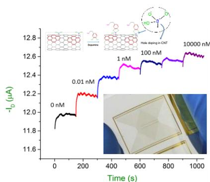
Figure. High-sensitivity detection of dopamine by biosensor based on pyrene-1-boronic-acid-decorated CNT TFT
