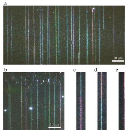
Fig. 2. True color imaging of SWCNTs. a, b, Typical true color image of horizontally aligned SWCNTs on Si wafer with 100 nm SiO<sub>2</sub>. c-e, Typical true color images of three individual SWCNTs with intramolecular junctions.
