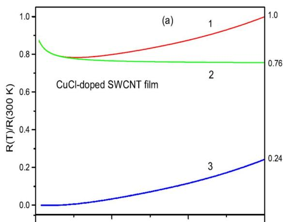
Fig.2. The electrical resistance of CuCl@SWCNT film. (1) experimental data, (2) tunneling between nanotubes, (3) nanotube contribution.
