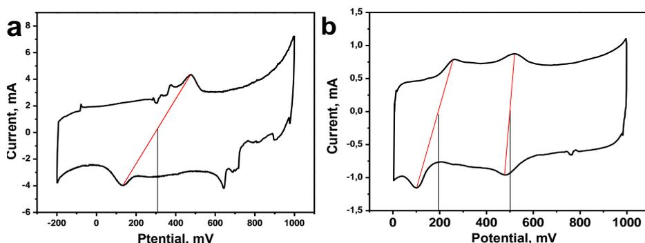
**Fig. 1.** Cyclic voltammograms of double-layered carbon nanotubes after oxidative treatment with mineral acids (a) and multiwall carbon nanotubes after hydrothermal treatment (b). The peaks on the CV curves correspond to the oxidation and reduction processes of oxygen-containing functional groups
