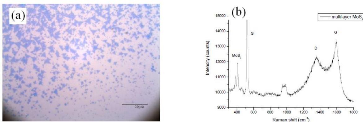
Fig.1. (a) Optical image of MoS<sub>2</sub> on SiO<sub>2</sub>/Si substrate; (b) Raman spectra of multilayer MoS<sub>2</sub> film grown on transferred CVD graphene.
