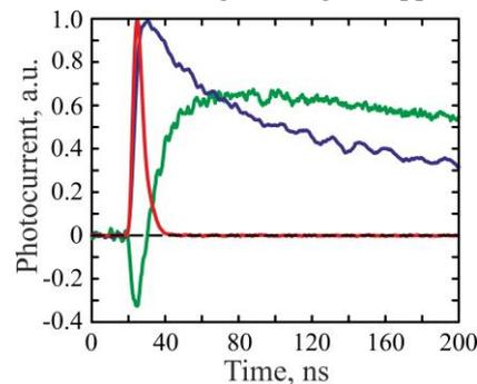
Fig. 1. Oscillograms of the photocurrent pulses induced by *s*-polarized (blue line) and the *p*-polarized (green line) laser beam. Red line shows temporal profile of the excitation laser pulse at 2000 nm.
