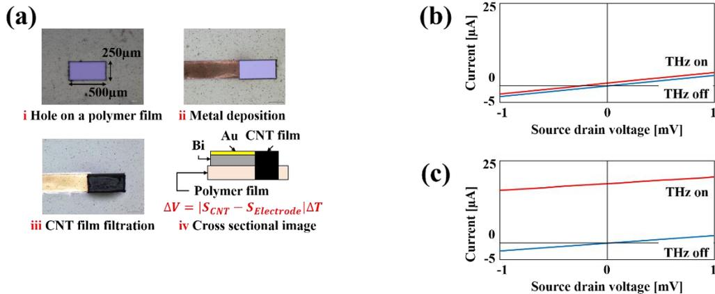
Fig.1 (a) Optical images of fabrication processes and schematic image of the present device structure. (b) Current-voltage characteristic of the conventional device under 29-THz irradiation. (c) Current-voltage characteristic of the present device under 29-THz irradiation.
