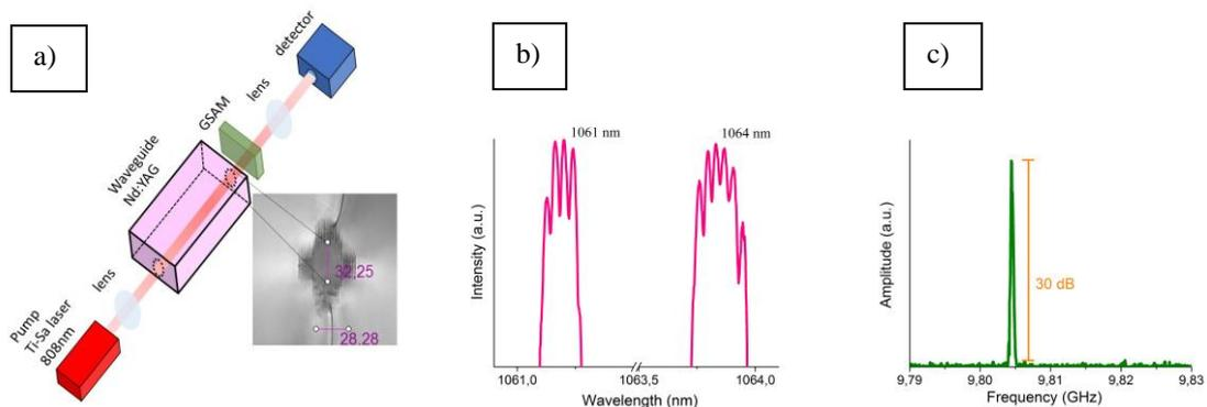
Fig.1. (a) The scheme of the waveguide Nd:YAG laser and obtained optical (b) and RF spectra (c)
