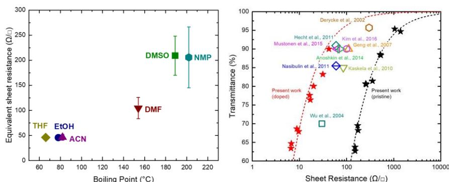
**Figure 1.** a) The resulting equivalent sheet resistance of the HAuCl<sub>4</sub>-doped samples at RT plotted vs. the boiling temperature of the solvents. b) Comparison of the performance of SWCNT-based TCFs after p-type doping: sheet resistance vs. optical transparency at 550 nm. Dashed lines indicated theoretical relationship between transmittance and sheet resistance of pristine (black) and HAuCl<sub>4</sub>-doped (using EtOH as a solvent) SWCNT films (red) obtained in this work.
