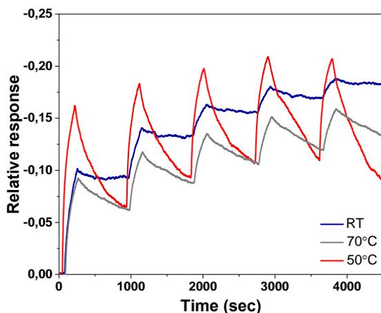
Fig. 1. Cycle-by-cycle response of fluorinated DWCNTs against 100 ppm of NO<sub>2</sub>, measured at room temperature (RT) and enhanced temperatures.
