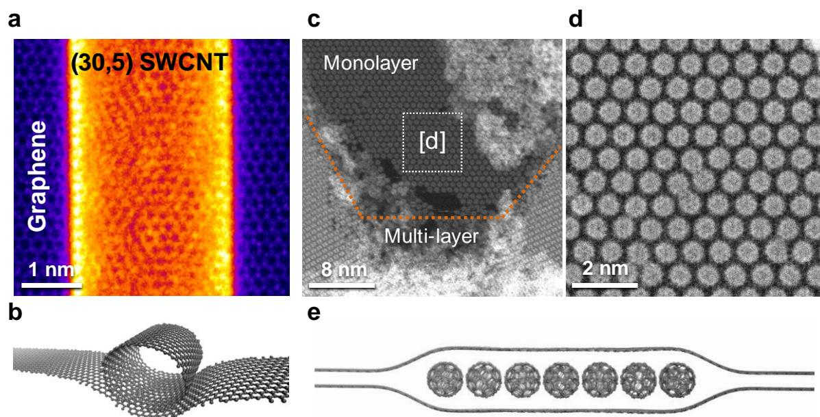
Fig. 1 a) A (30,5) SWCNT suspended on graphene and b) the recovered 3D structure of the molecular pair. c) An overview of a buckyball sandwich showing both mono- and multi-layer regions and d) an atomically resolved magnification of the monolayer and finally in e) a simulated sandwich structure.
